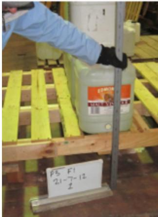
Fielding measuring displacement under load.
